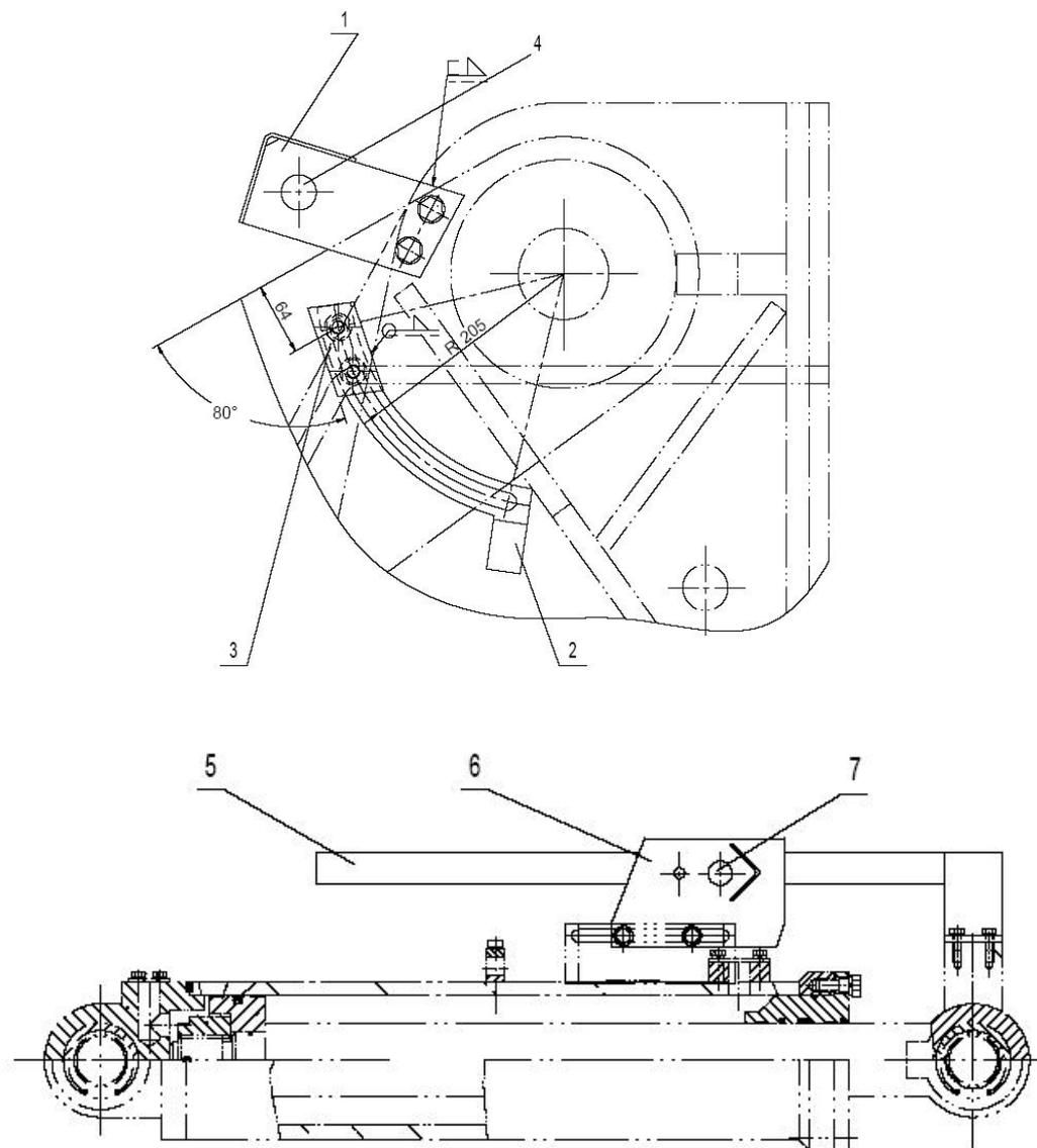
举升限位和自动放平机构 LIFTING LIMIT AND BUCKET AUTO-LEVELING
