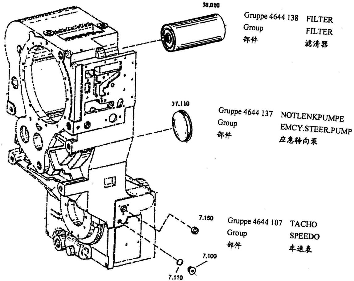
滤清器, 应急转向泵, 车速表 FILTER, EMERGENCY STEERING PUMP, SPEEDOMETER
